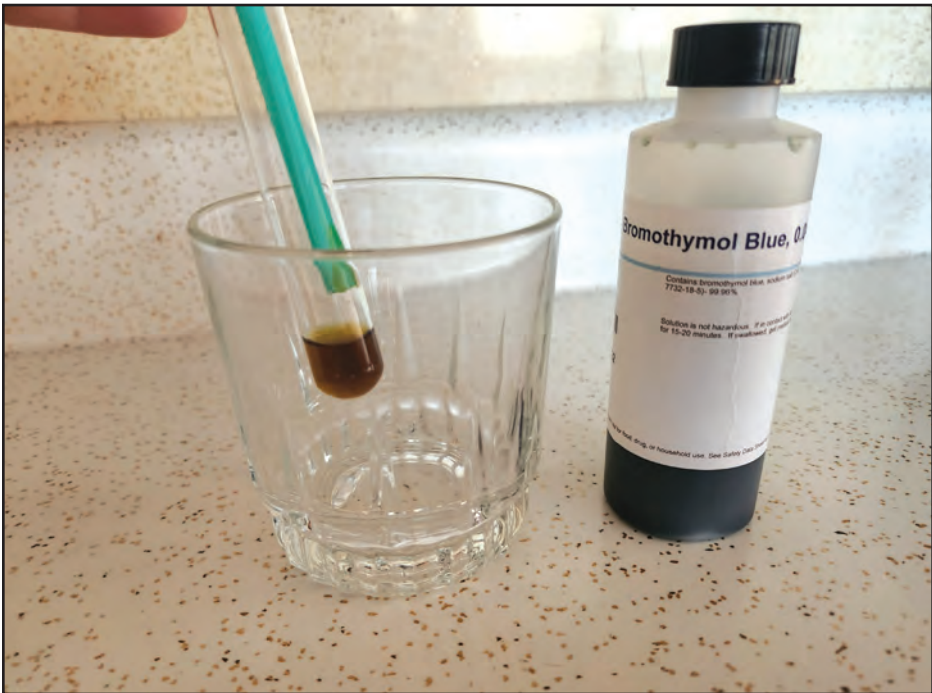
BTB in test tube with straw after being exposed to CO2.
