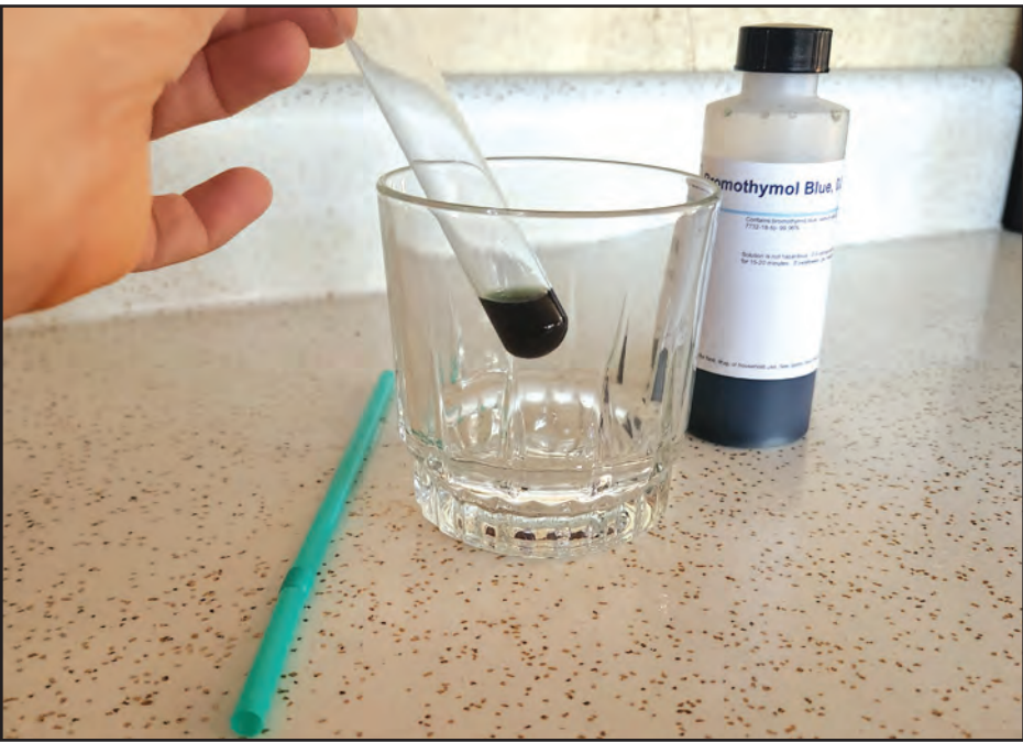
Bromothymol blue (BTB) in test tube before being exposed to CO2.
